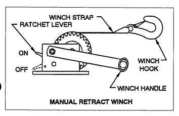
Slowly winch the room in by turning the WINCH HAN-DLE clockwise. The RATCHET LEVER should produce a loud sharp clicking noise.
