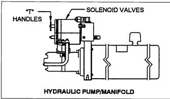
Open the SOLENOID VALVES by turning the "T" HANDLES counterclockwise.
