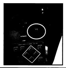
Your vehicle is equipped with an emergency start switch, located on the dashboard. This switch allows you to switch to the coach battery to start the engine in the event of a low chassis battery. To activate the emergency start, push and hold in the emergency switch, then start the engine. Once the engine has started, release the switch.
