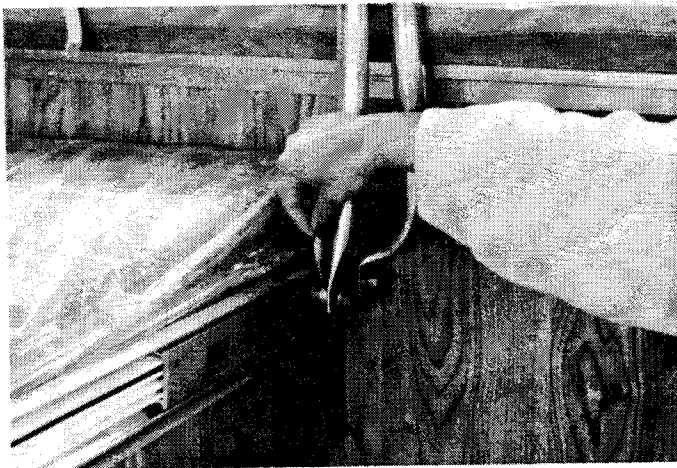
Step 3: Put down safety latch on left system bar, to secure roof. Located front of bunk on right side.
