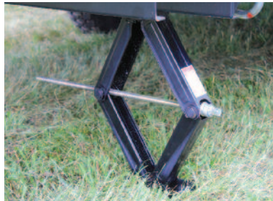
The four heavy duty scissor-style stabilizing jacks extend and retract easily using a cordless drill and the Canimex drill bit.
