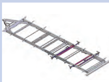
Norco NXG chassis featuring E-Coat technology
