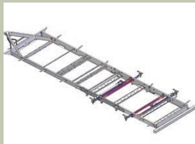
Norco NXG chassis featuring E-Coat technology
