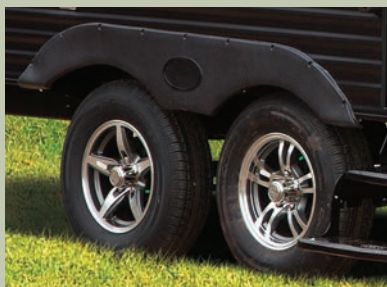
Tandem axles enhance stability
