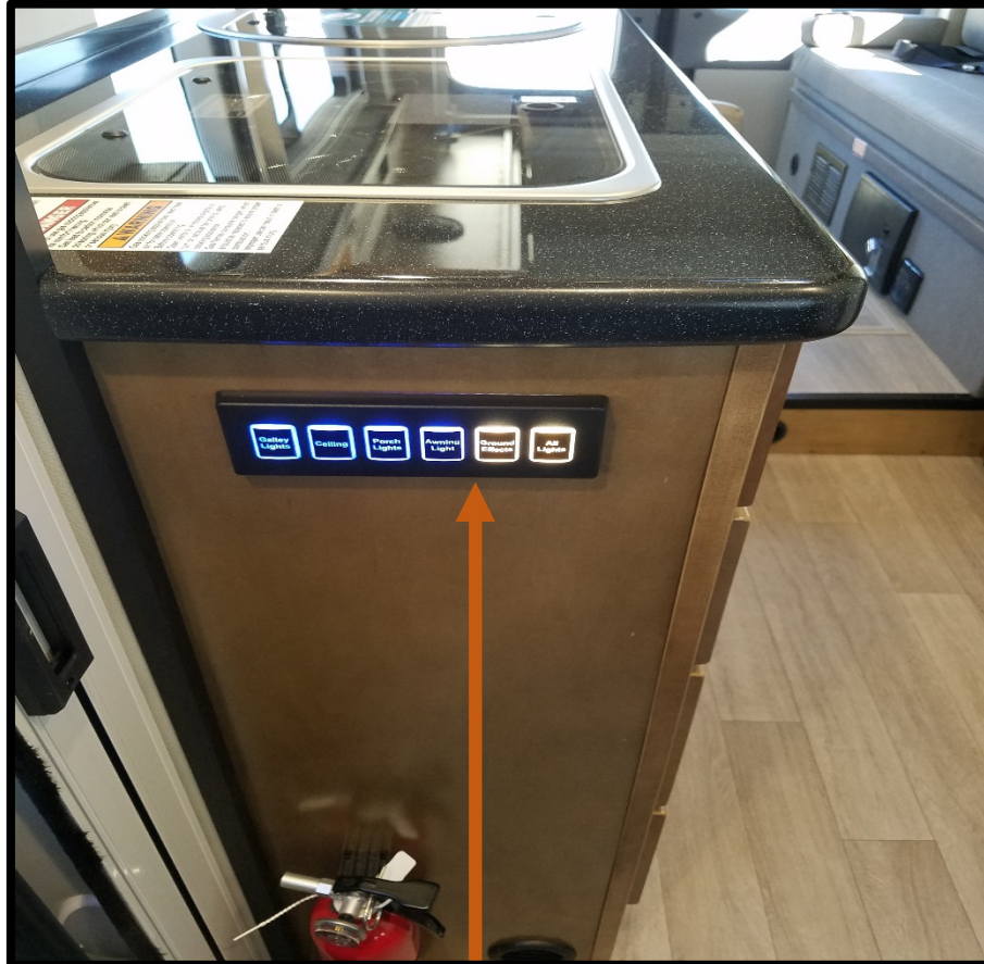
Multi-Plex Panel Located Right as you Enter/Exit Individually Controls All Lighting Zones (2) Locations / No Switches to Search For!
