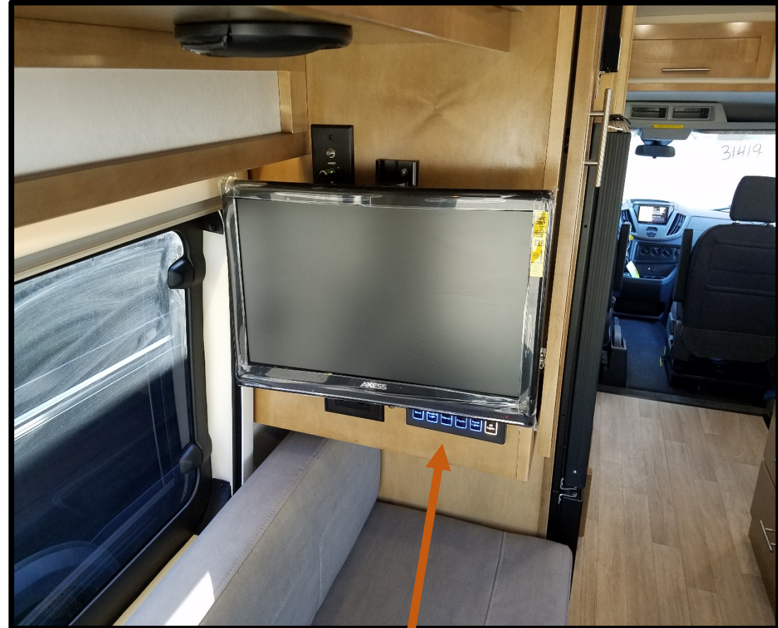
2 nd Multi-Plex Panel at TV/Bed for Easy Access to All Lighting Functions while Sleeping
