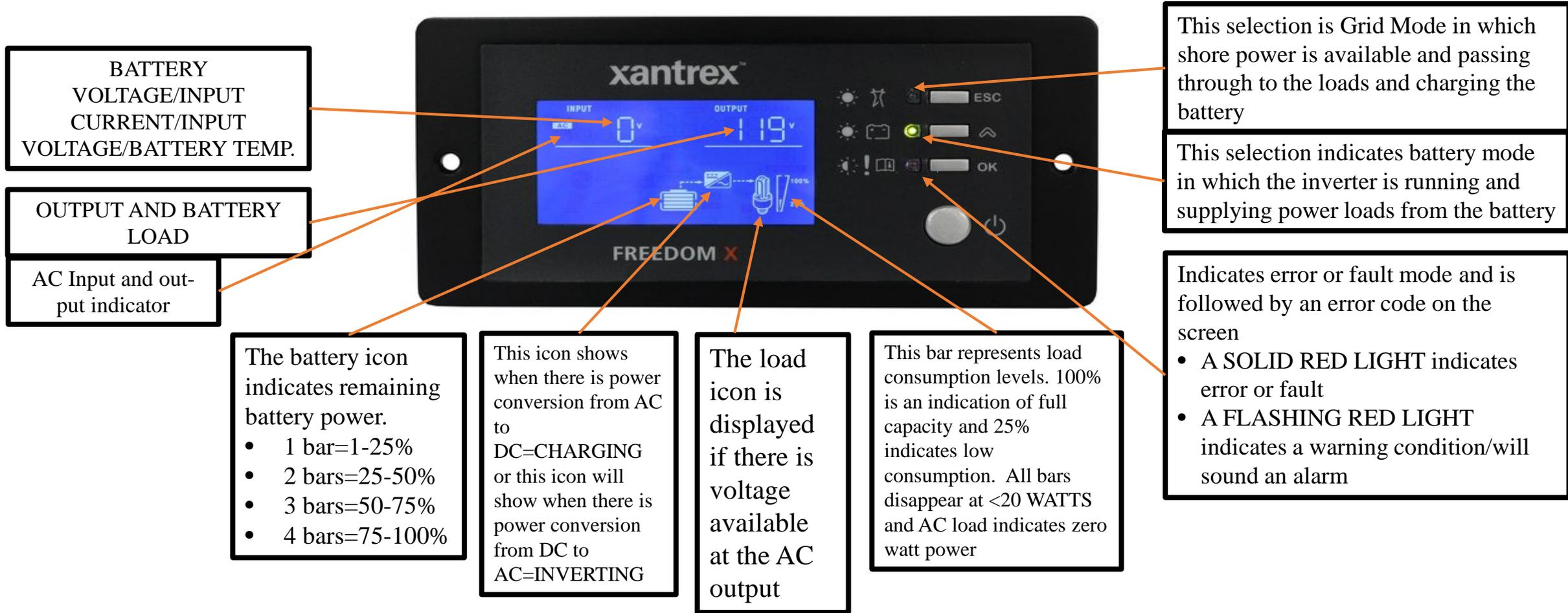
The Freedom X Remote Panel for your Xantrex Invertor Charger enables you to control and monitor the invertor from a convenient location and read important power supply information.
