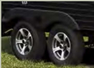
Tandem axles enhance stability
